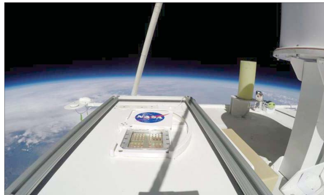
The picture shows MARSBox payload in the Earth's middle stratosphere (38km altitude). The shutter is open exposing the top layer samples to UV radiation.
